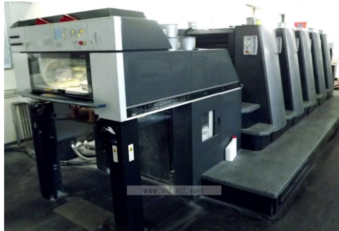
Abb. 9: Bogenoffsetmaschine Speedmaster CD 74-5 18
